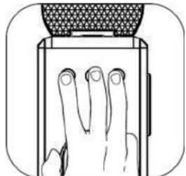
In power save mode, press and hold three buttons simultaneously for 3 seconds. After the buzzer sounds and three buttons blink 5 times, the machine will be set to room temperature water mode, and the boiler will stop heating.
