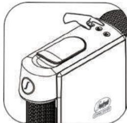
In power save mode, press and hold the Espresso button for 3 seconds; the machine will enter the water quality selection function. Press the Espresso button once to reduce the water quality level one level, press twice to reduce one more level and so on. Press the Lungo button to increase the level (total 5 levels).
