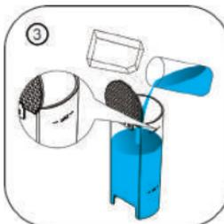
Put in the descaling agent in accordance with the instructions and mix with water; fill the water tank up to the MAX.
