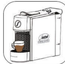
Press the Medium button; after buzzer sounds, 40ml coffee brewed. Buzzer sounds 2 seconds after pump stops, meaning brew completed. (Medium button blinks once per sec.; other buttons stay on).
