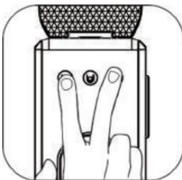
In standby mode, press and hold the Espresso and Lungo buttons for 3 seconds, buzzer sounds and machine enters into power save/switch off mode.
