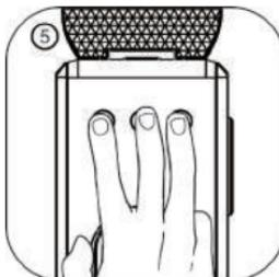
To enter the descaling mode, with the machine in standby mode, press both the Espresso, Medium and Lungo buttons for 3 seconds.
