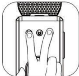
In power save mode, press the Espresso and Lungo buttons simultaneously for 3 seconds; after buzzer sounds, machine enters temperature setting mode.
