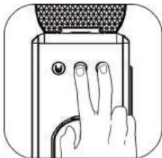
In standby mode, press and hold the Lungo and Medium buttons for 3 seconds; the machine will enter volume setting. After the buzzer sounds, the three buttons blink simultaneously.
