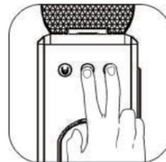
Press and hold the Lungo and Medium buttons for 3 seconds. When the buzzer sounds, this means the set volume is saved.
