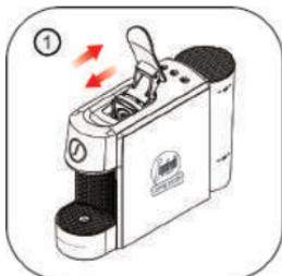
Lift and close the lever to eject the capsule into the used capsule container.
