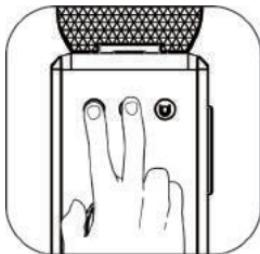
In power save mode, press Espresso and Medium button to empty the machine.
