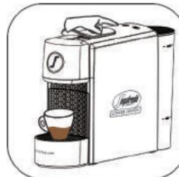
Press the Espresso button; after buzzer sounds, 25ml of coffee is brewed. Buzzer sounds 2 seconds after pump stops, meaning brew completed. (Espresso button blinks once per sec.; other buttons stay on).
